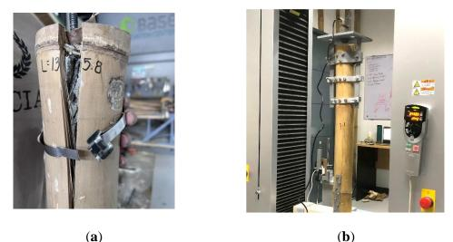
**Fig. 11**. Sample testing of foundation connection: (a) failure mode of embedded rebar; (b) tensile test for steel plate connections.
