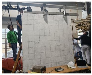
**Fig. 12**. Reaction frame with the dynamic actuator (BIC).
